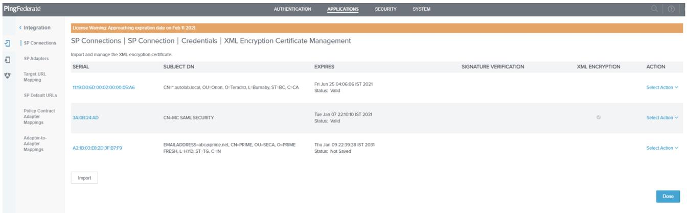
11. On the Select XML Encryption Certificate tab of the *Credentials* page, select the **AES-256** and **RSA-OAEP** radio buttons, then select the uploaded certificate from the drop-down list and click **Next**.
